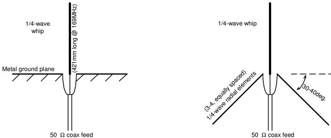
Fig.5: Quarter wave antenna / ground plane configurations
