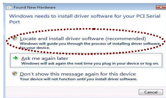
12. If "PCI Serial Port" has been successfully installed, "Found New Hardware" Message box will appear. Click "Locate and install driver software (recommended)".
