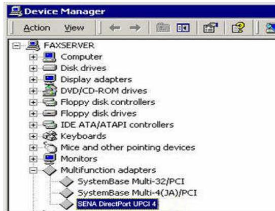
12. After all installations are completed, you can check the device information in [Setting]→ [Control Panel]→ [System]→ [Hardware]→ [Device Manager]. You can see the SENA DirectPort UPCI installed at “Multifunction adapters” category and “DirectPort UPCI – Serial Port” at “Ports (COM & LPT)” category in device manager.
