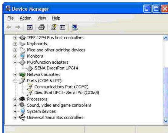
9. After a successful installation, “SENA DirectPort” can be seen under “Multifunction adapters” and “DirectPort UPCI – Serial Port” can be seen under “Ports (COM & LPT)” in device manager.
