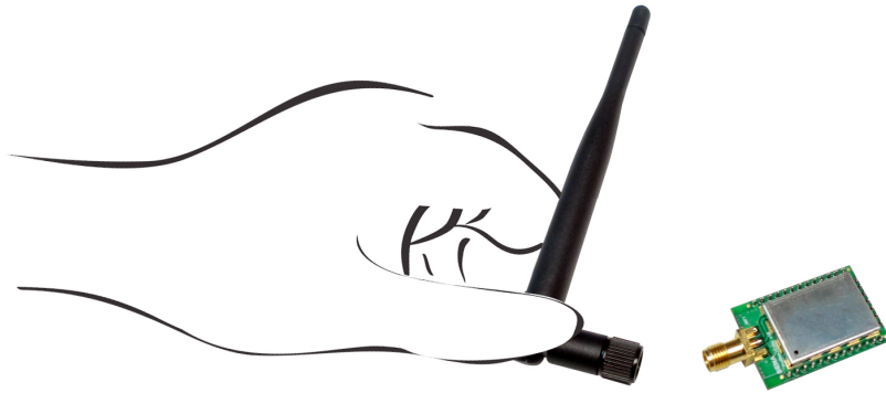
Figure 2-2 RP-SMA Dipole Antenna Installation
