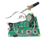
③ Connect Power supply to Jig Board
