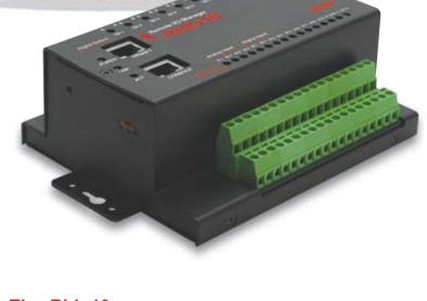
**The Rhio10,** Remote I/O Manager is simple and easy-to-use Ethernet Data Acquisition System that communicates with PCs and other computers over Ethernet and Internet networks. They utilize the open systems environment of Ethernet to acquire data from any number of remote locations.
