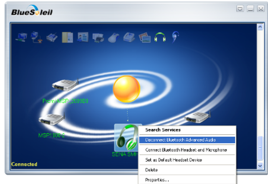
Figure 3.22: Disconnection Bluetooth Advanced Audio
