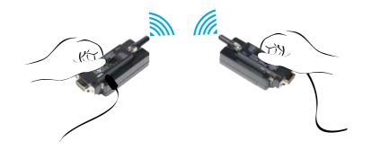
Parani-SD provides Pairing Button for instant configuration without a PC to make an automatic connection between two Parani-SDs. (Two Parani-SDs as SD1 and SD2, respectively.)
